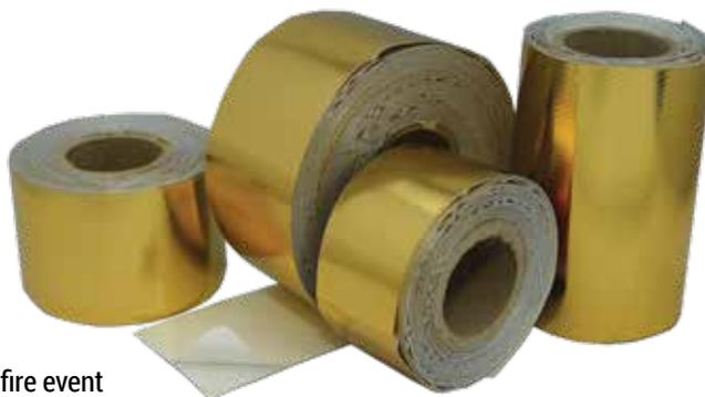
Cold-Gold Tape™ won't degrade after long-term heat exposure. It can take constant ambient temps of up to 1,100 degrees Fahrenheit, intermittent ambient temps of 2,000 degrees Fahrenheit. While Cold-Gold Tape™ is not *designed for direct heat contact* it can shield over 90 percent of radiant heat with a 1 inch space from the heat source.
