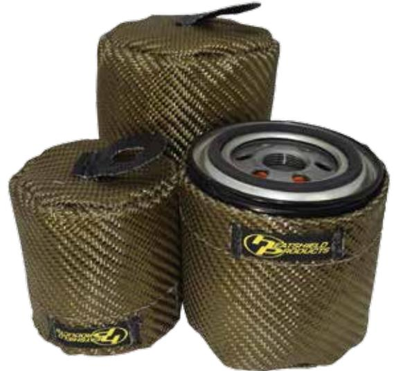
High heat generated by the exhaust system can saturate the oil filter, which adversely affects the temperature of the oil running through the filter, as well as the filter internals. In addition, the usual mounting location of the oil filter exposes it to road debris that gets kicked up under the vehicle and can potentially puncture the filter, cause oil loss and engine failure. Lava Oil Filter Shield™ protects the oil filter from heat and road debris.
